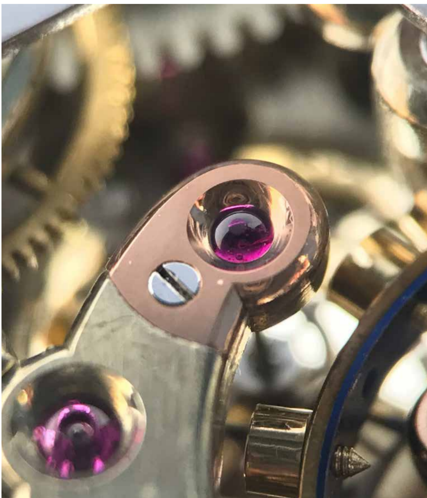
A gold end-piece for the escapewheel pinion limiting the vertical play and pivot friction, as with a balance wheel pivot.
